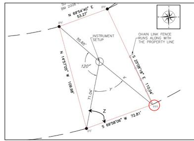
having trouble finding the final corner due to the chain link fence that follows the property line. The metal detector has been less effective since there is so much metal in the area.
